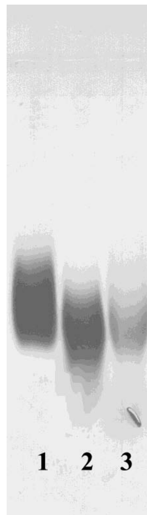
Figure 1. Agarose gel electrophoresis (in the absence of SDS) of nonmodified and succinylated WPI aggregates. Proteins were stained according to the standard Coomassie brilliant blue staining method: lane 1, nonmodified WPI-aggregates; lane 2, 56% succinylated WPI-aggregates; lane 3, 93% succinylated WPI aggregates.
